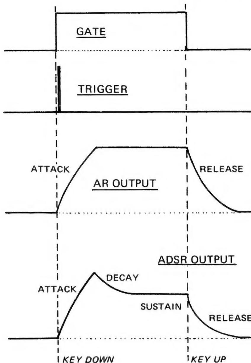
NOTE: The ADSR is initiated with a gate and trigger voltage, and the AR envelope requires only the gate.
