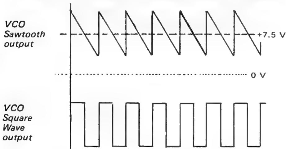
the point at which the comparator switches. When the pulse width sliders on the front panel are at minimum, the comparator will switch exactly in the middle of the sawtooth slope, producing a square wave (50% duty cycle). The output of the comparator (Z3, pin 8) is processed through Z4A which inverts the shapes of the pulse output.
